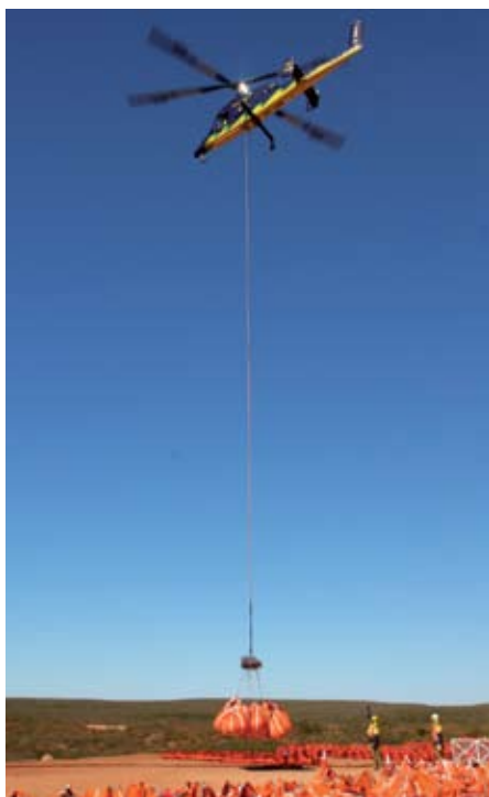
K-MAX helicopter transports seismic equipment to reduce impact on the Barrow Island environment.
