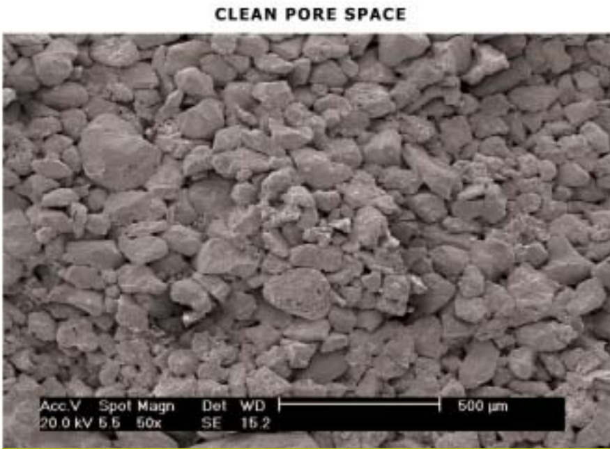
Figure 13-12: Photo-micrograph Showing Clean Pore Space
