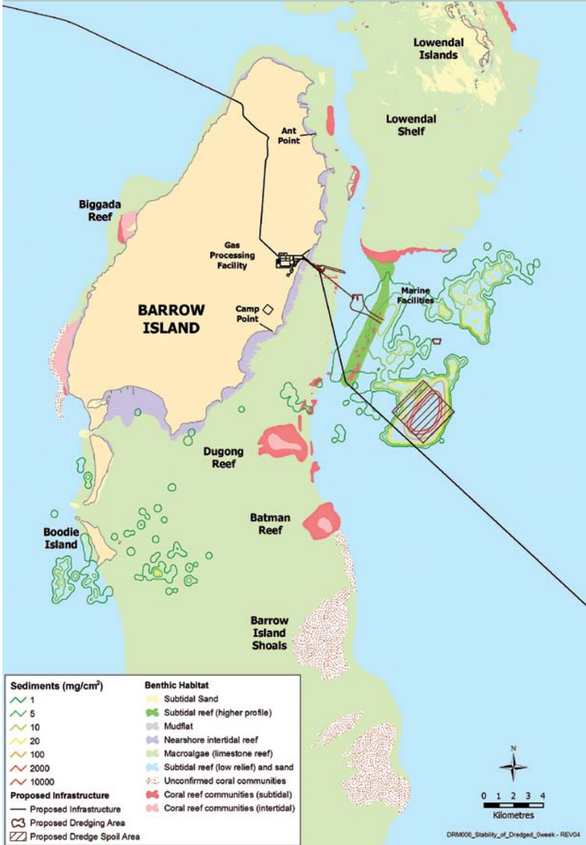
Figure 10: The Anticipated On Bottom Sediment Load at the End of Dredging (0 Weeks)
