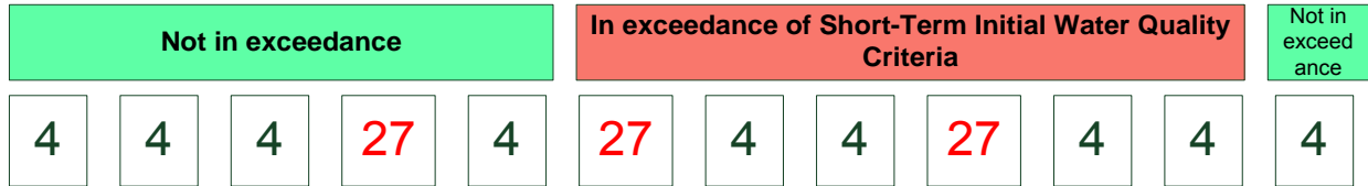
Figure 2 Exceedances of Daily Median TSS (25 mg/L) Threshold Concentrations and Exceedances of the Short-term Initial Water Quality Criterion ( \geq 25 mg/L for 2 days in a 6-day period)
