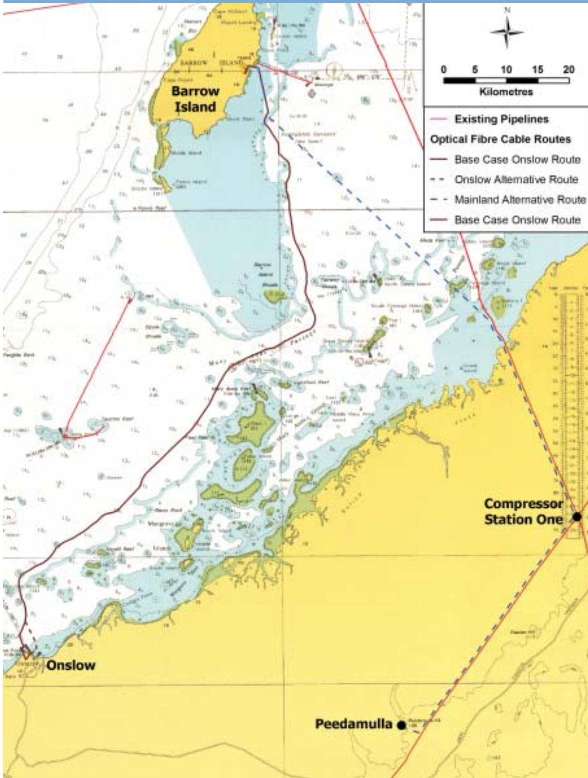
Figure 6-18: Possible Routes for Optical Fibre Communications Link
