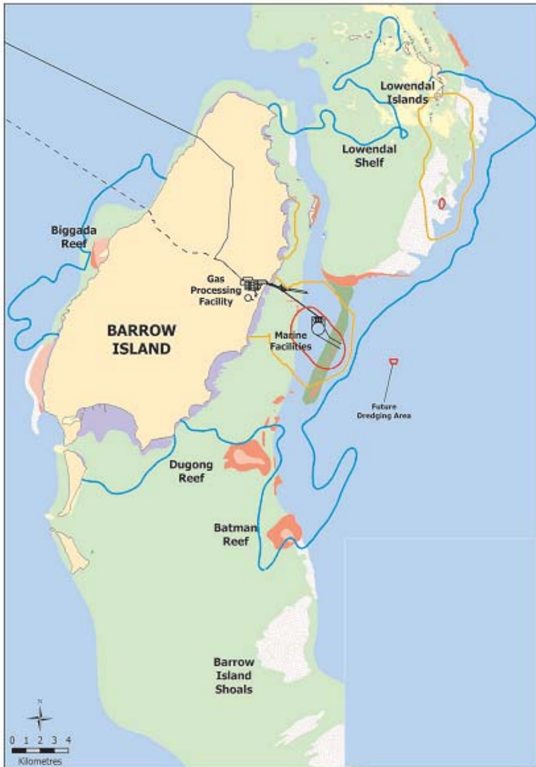
Figure 7.4: Mortality zones derived from TSS data for the “Base” case. Level 1 (red) = high impact, Level 2 (orange) = moderate impact, Level 3 (blue) = visible plume (exposure above 2mg/litre).
